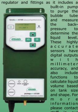
built-in pump to purge the bubble tube and measure backpressure to determine the liquid level. These highly accurate sensors have digital outputs with millimeter accuracy, and also include functions to calculate liquid volume based on tank size and shape. For m o r e information please contact staff in our Environmental group.
