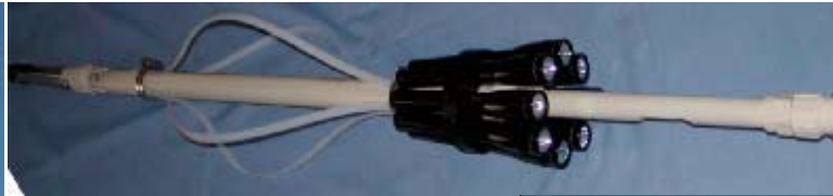
The Super 8 Light and Adjustable Super 8 Light provide supplemental light for use in boreholes, shafts, mines, and caves. Versatile brackets allow these lights to be attached at many different places on the GeoVISION™ system. Supplemental off camera light also improves the quality of the image by increasing the subject texture and by reducing glare. The two Super 8 Lights are bright and are recommended for large boreholes, shafts, and mines.
