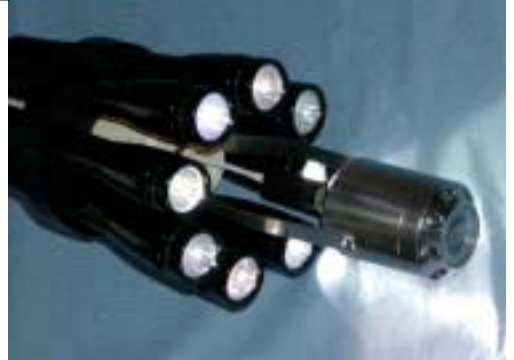
The Super 8 Light and Adjustable Super 8 Light provide supplemental light for use in boreholes, shafts, mines, and caves. Versatile brackets allow these lights to be attached at many different places on the GeoVISION™ system. Supplemental off camera light also improves the quality of the image by increasing the subject texture and by reducing glare. The two Super 8 Lights are bright and are recommended for large boreholes, shafts, and mines.
