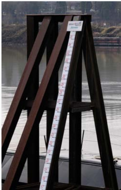
Custom Stevens staff gage mounted on a sloped pier on the Willamette River in Portland, Oregon. The submarine pictured is the USS Blueback.
