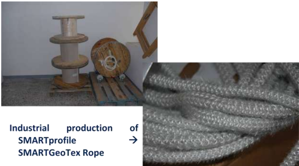
Figure 7 – Production of sensing cable clad in SMARTGeoTex Rope
