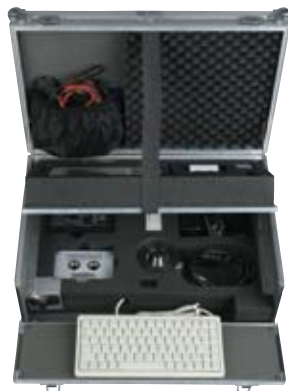
Measurement case level 2 with measuring head, accumulator, load cell, charger, PC-keyboard with protective foil
