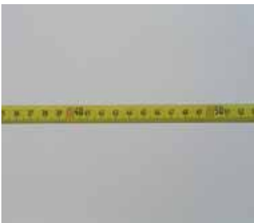
BFM cable with graduation at 1 mm intervals
