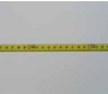
BFM cable with graduation at 1 mm intervals
