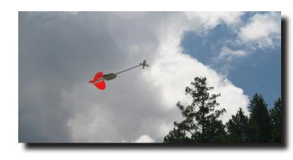
The Anasphere SmartTether represents a revolutionary approach to gathering atmospheric profiles within the lower troposphere using tethered blimps, balloons, or kites. It is orders of magnitude faster and less expensive as compared to traditional tethersonde systems and allows users to collect data simultaneously at multiple points along a tether. SmartTether applications include boundary layer wind profiling, fire weather, pollution monitoring, emergency response and flux measurements.
