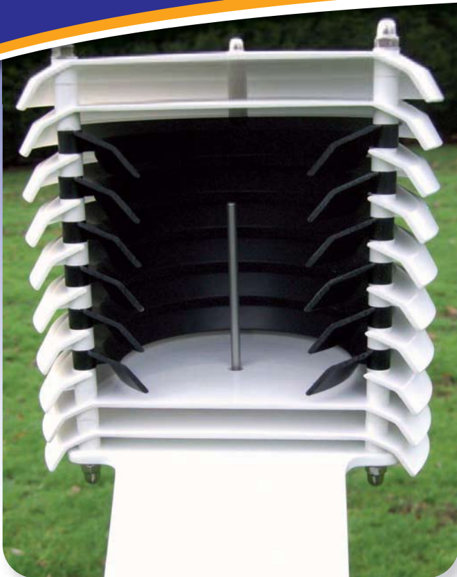
A cross-sectional cutaway showing the external and internal louvers of a RAD 01 shield
