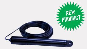
The ES&S 1500 Electrical Conductivity sensor is designed for measuring electrical conductivity of liquids at remote locations. It is specifically suited for low power water quality applications where access and site visits are limited. Unlike conventional electrode based cells, the encapsulated toroid design requires very little maintenance, ensuring many years of accurate data collection without recalibration and without deterioration of metals.
